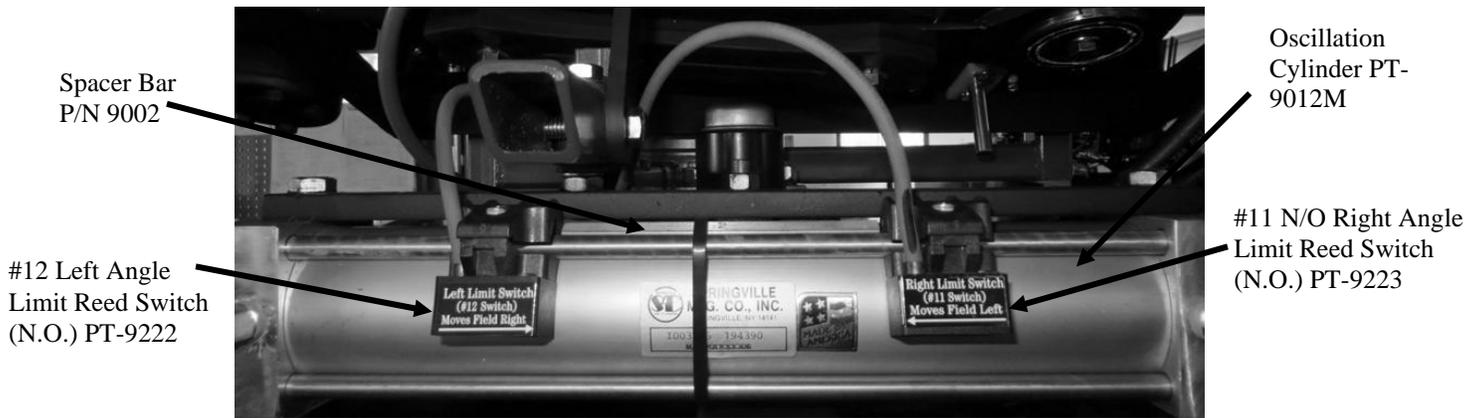
**Pat-Trap® #12 & #11 Limit Reed Switches on Oscillation Cylinder**
